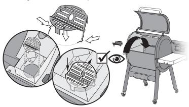
Check that the glow plug is fully seated in the shuttle against the grounding tab. After it is installed, make sure the glow plug is visible through the fuel grate.
