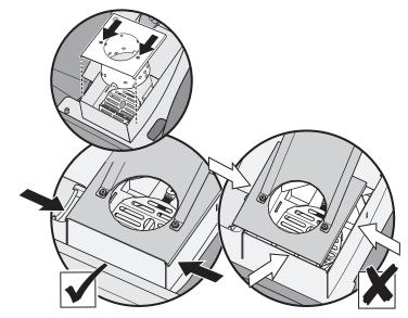
Check that the front and back Flavorizer brackets are pushed all the way down on their mounting tabs and the pellet slide is positioned under the Flavorizer bracket.
